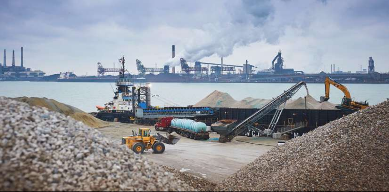
The Huron Spirit features a 150-ft self-unloading boom ideal for efficient discharge of bulk commodities. Here it is pictured unloading aggregates at the Port of Monroe.
