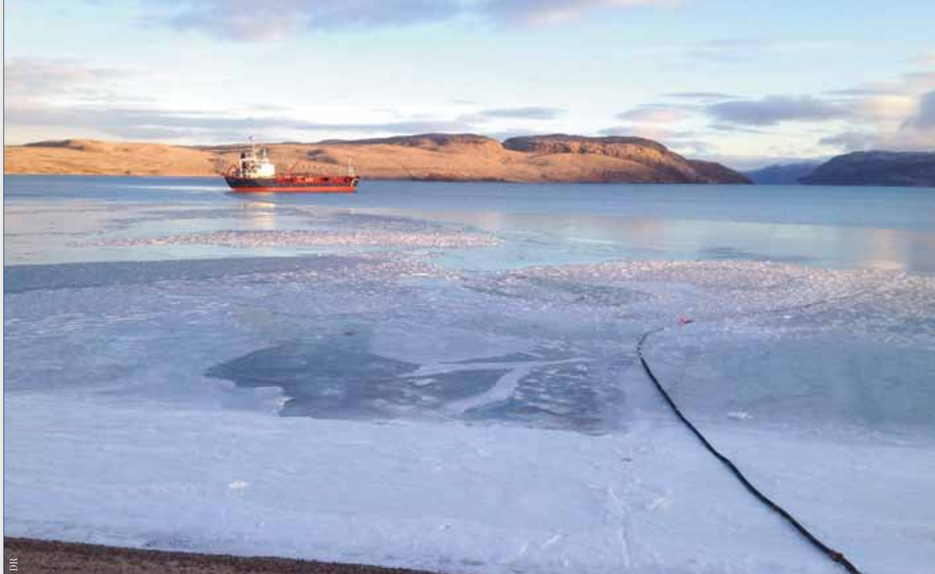
Hoses transmitting fuel to a beach location can vary in length between 2,400 ft and 7,500 ft.
