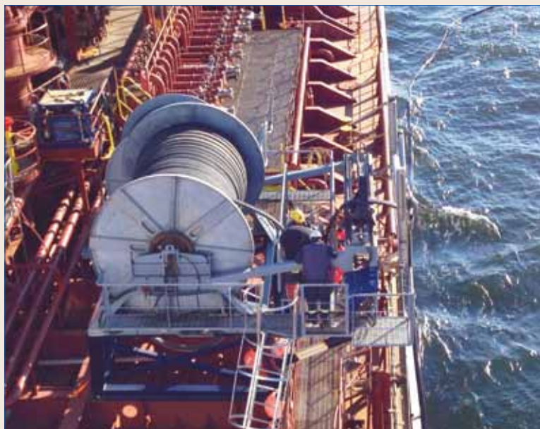
Crew help to run hose for service from a special reel aboard ship.
